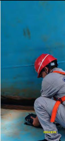
A photograph showing a worker in safety gear (red hard hat, safety harness) performing ultrasonic testing on a blue steel structure. The worker is kneeling and using a device. The date '2024/8/24' is printed in the bottom right corner of the image.                                                               |
